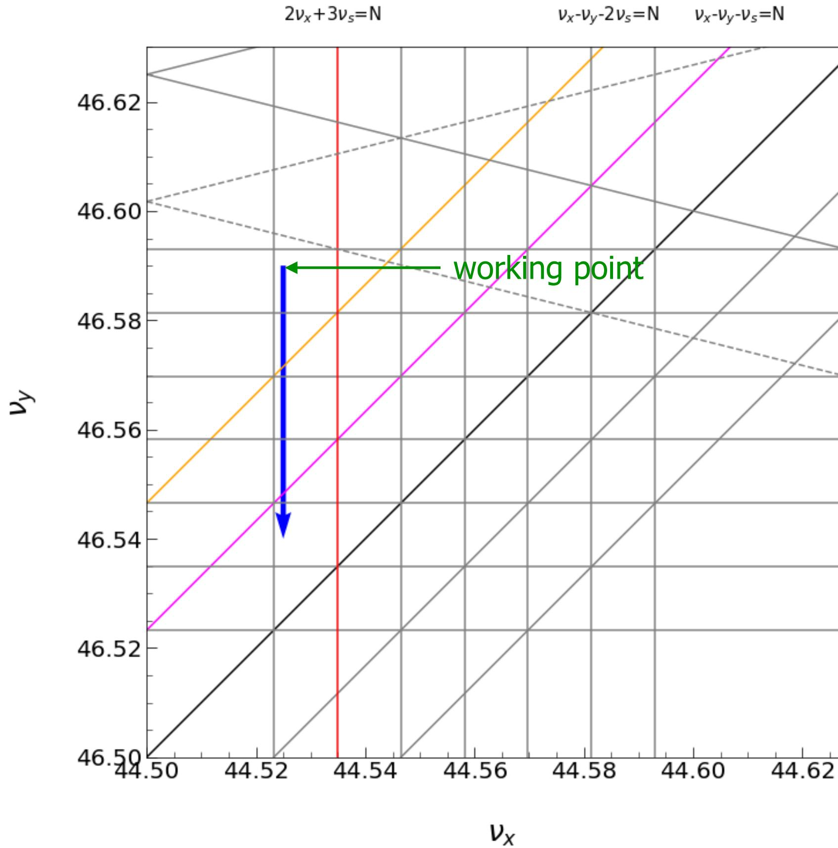
The rotatable sextupoles (6 families for right and left side of IP) are used to make the first synchro-beta coupling resonance weak together with the second resonance.
