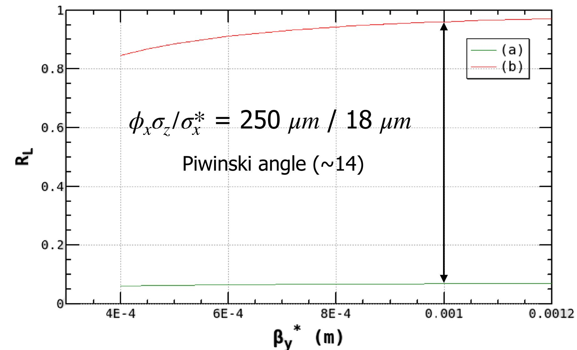
In the case of  $\beta_y^*$  is 1 mm, the luminosity loss is 4 %.
