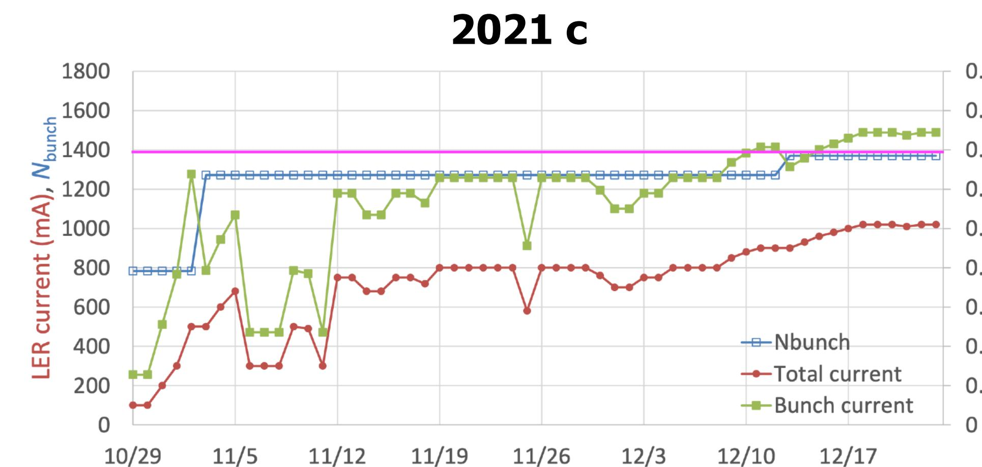
Bunch current was smaller than 0.7 mA in the most of operation time
