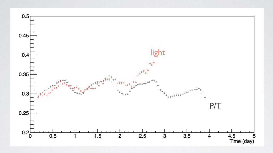
Together with the increasing behavior, there is a clear correlation with the gas density (P/T) that seems not visible in the current;
