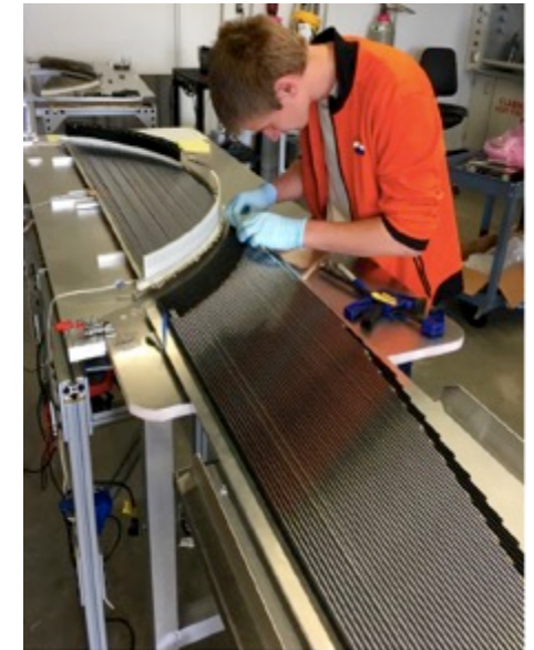
Panel: Straw Installation
