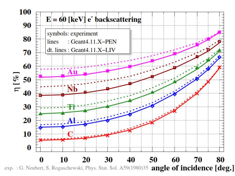
Penelope ionisation below 100 keV allows reproduce backscattering of electrons with higher accuracy as it was in Geant4 10.6
