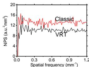
Figure 2: NPS of flood illumination of the detector for classical code and for VRT.
