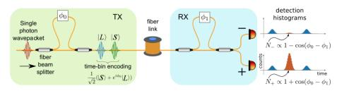
Time-bin is robust in fiber-optic propagation!
