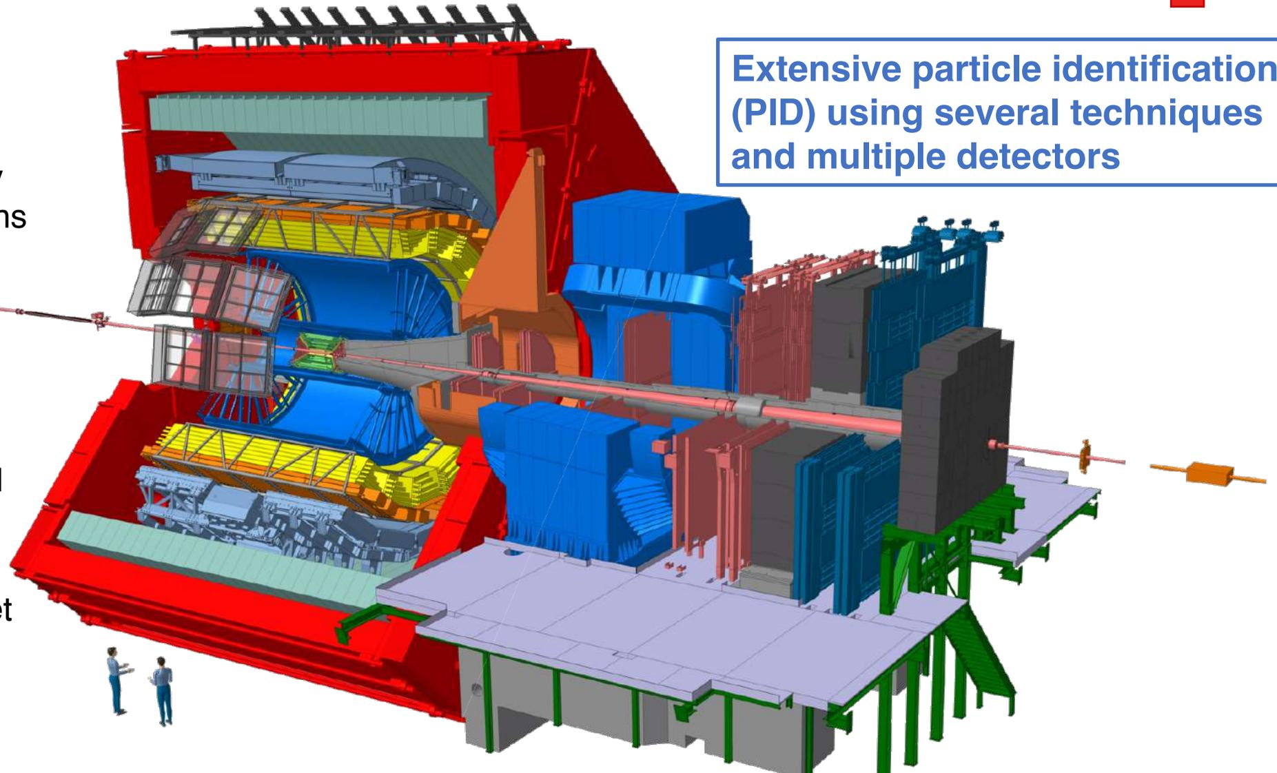
Extensive particle identification (PID) using several techniques and multiple detectors
