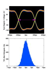
Measurement of jitter rejection on a 5.12 GHz LC-PLL designed at INFN Torino
