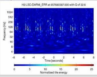
Multiple-bounce fringe wrapping event. Characteristic time-frequency feature. Caused by O(10) bigger motion than usual.
