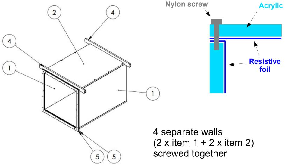
Double frame for cathode foil installation, screwed to the field cage
