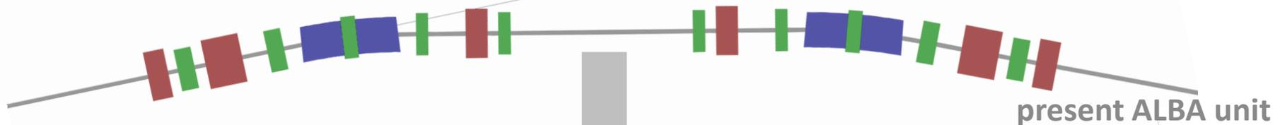
16 hybrid 7BA with anti-bend identical cells  $\rightarrow$  16 straights 4.35 m
