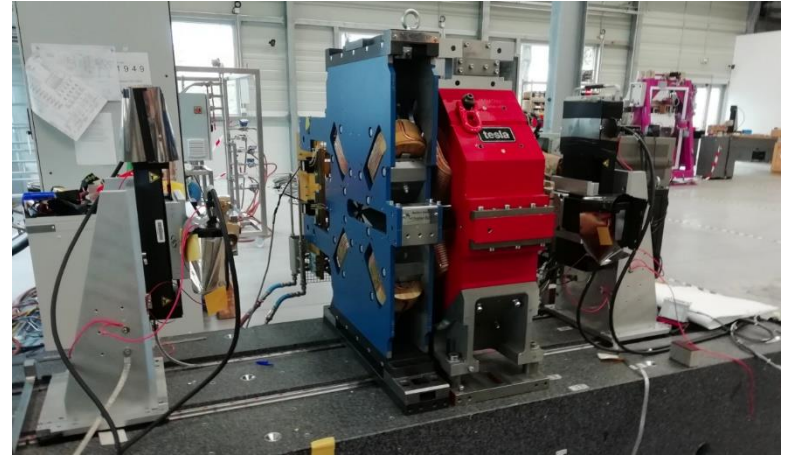
Octupole and quadrupole installed on a measurement bench
