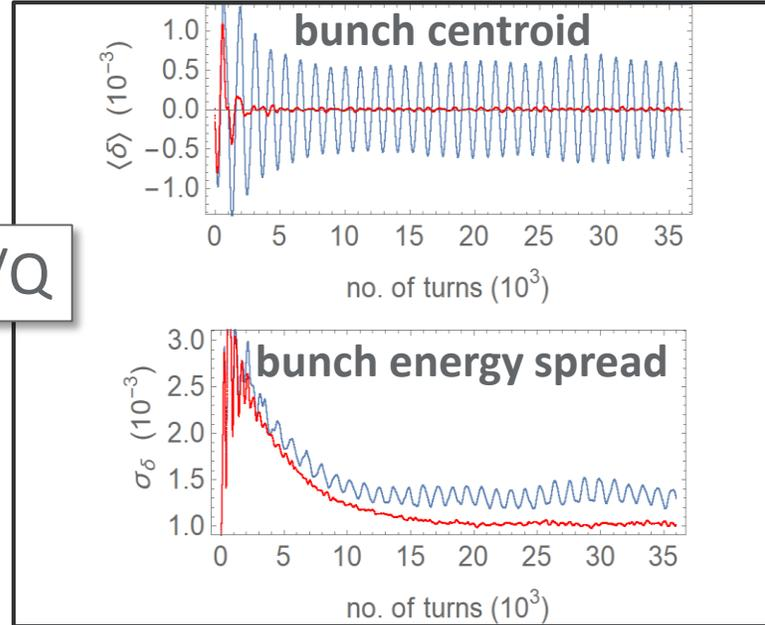
Steady-state oscillations settle in when overstretching
