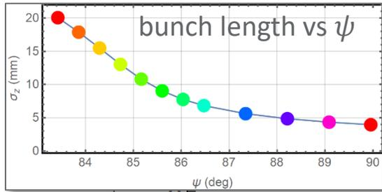
tuning angle for the bunch profile to develop two humps (vanishing rf voltage slope,  $V'_{rf} = 0$ ):
