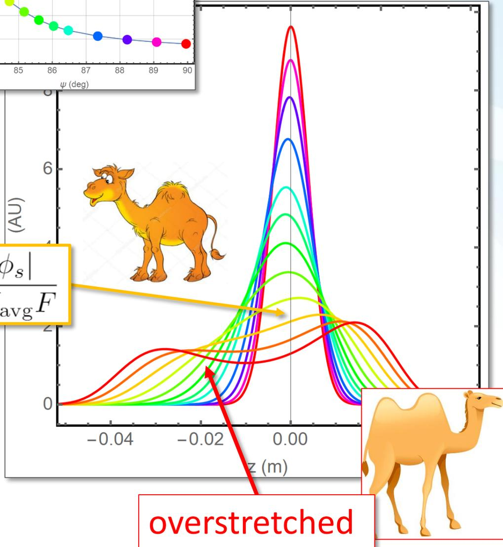
For  $\psi = \psi_{crit}$  and for a given current there's a special value of  $R_s$  such that  $V''_{rf} = 0$  as well  $\rightarrow$  quartic rf potential  $\rightarrow$  flat profile (often referred as "optimal")
