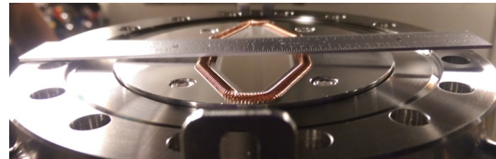
RF spring in a special groove
