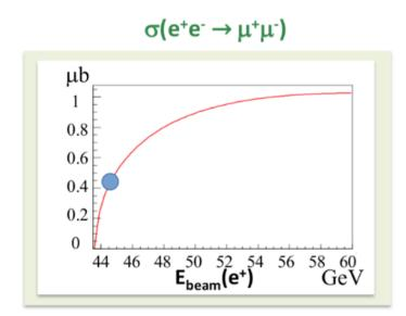
The value of sqrt(s) (*i.e.* E(e<sup>+</sup>) for atomic e<sup>-</sup> in target) has to maximize the muons production and minimize the beam angular divergence and energy spread
