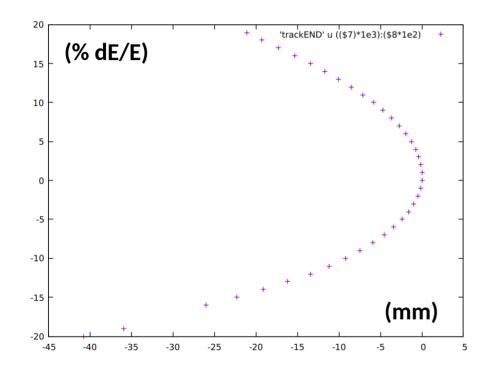
When reducing First Order Momentum Compation Factor to 10<sup>-4</sup>, Second order momentum compaction is not longer negligile factor limits the energy cannot be canceled in a single cell
