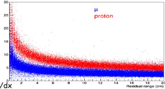
• First plot for the dE/dx vs range and for the particle identification test obtained for protons and muons.
