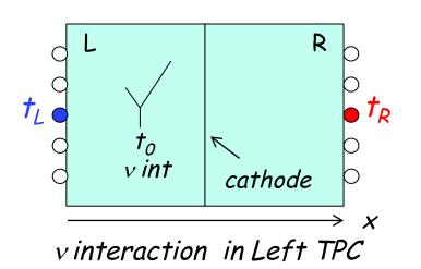
$\rightarrow$   $(t_L + t_R)/2$  provides a 1<sup>st</sup> evaluation of  $t_0 v$  interaction independent from v vertex position with  $\sigma \sim 2.4$  ns
