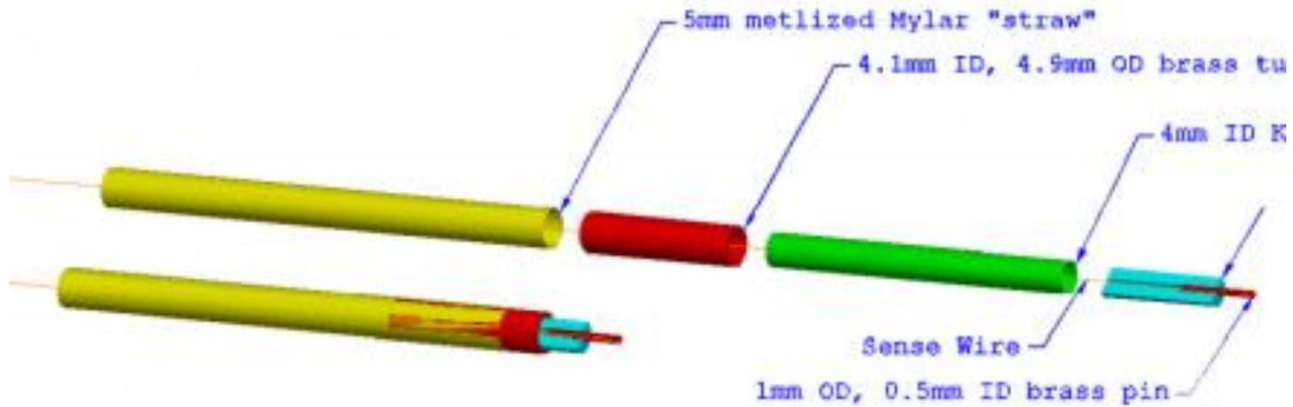
The detector has 23,000 straws distributed into 20 measurement stations across a 3 m length.
