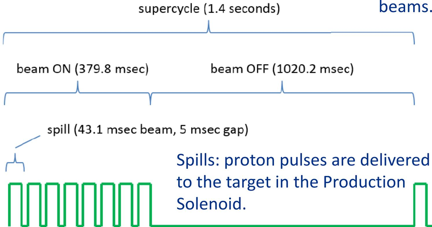
Each spill contains approximately 32 000 uBunches, for a total of 256 000 Bunches in a 1.4 second supercycle. A Bunch is 1695 ns.
