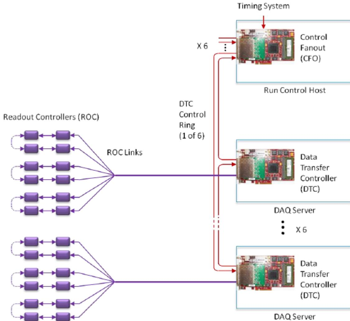
The Data Transfer Controller (DTC) collects data from multiple detector Readout Controllers.
