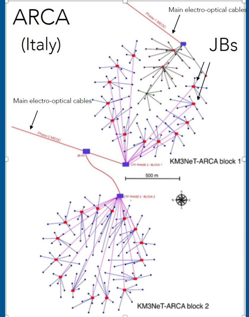
**ARCA is composed of 2 building blocks of 115 DUs** each with 90 m DU interspacing and 36m inter DOM spacing (0.5 km<sup>3</sup>=500Mton/block)
