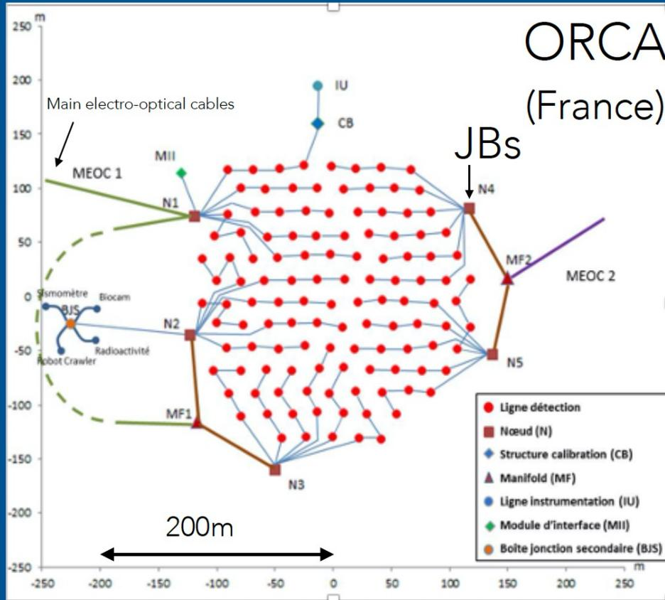
**ORCA is composed of 1 building block of 115 DUs** each with 20 m DU interspacing and 9m inter DOM spacing (7 Mton)
