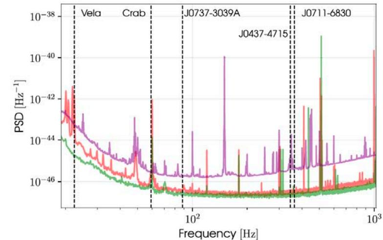
**Figure 1.** O3a noise PSD for H1, L1, and V1 shown in red, green, and purple. The H1 and L1 PSDs are calculated during a time period of optimal performance for the detector, while the Virgo PSD is averaged over the run. The vertical dashed lines indicate the searched frequency region for each of the five pulsars.
