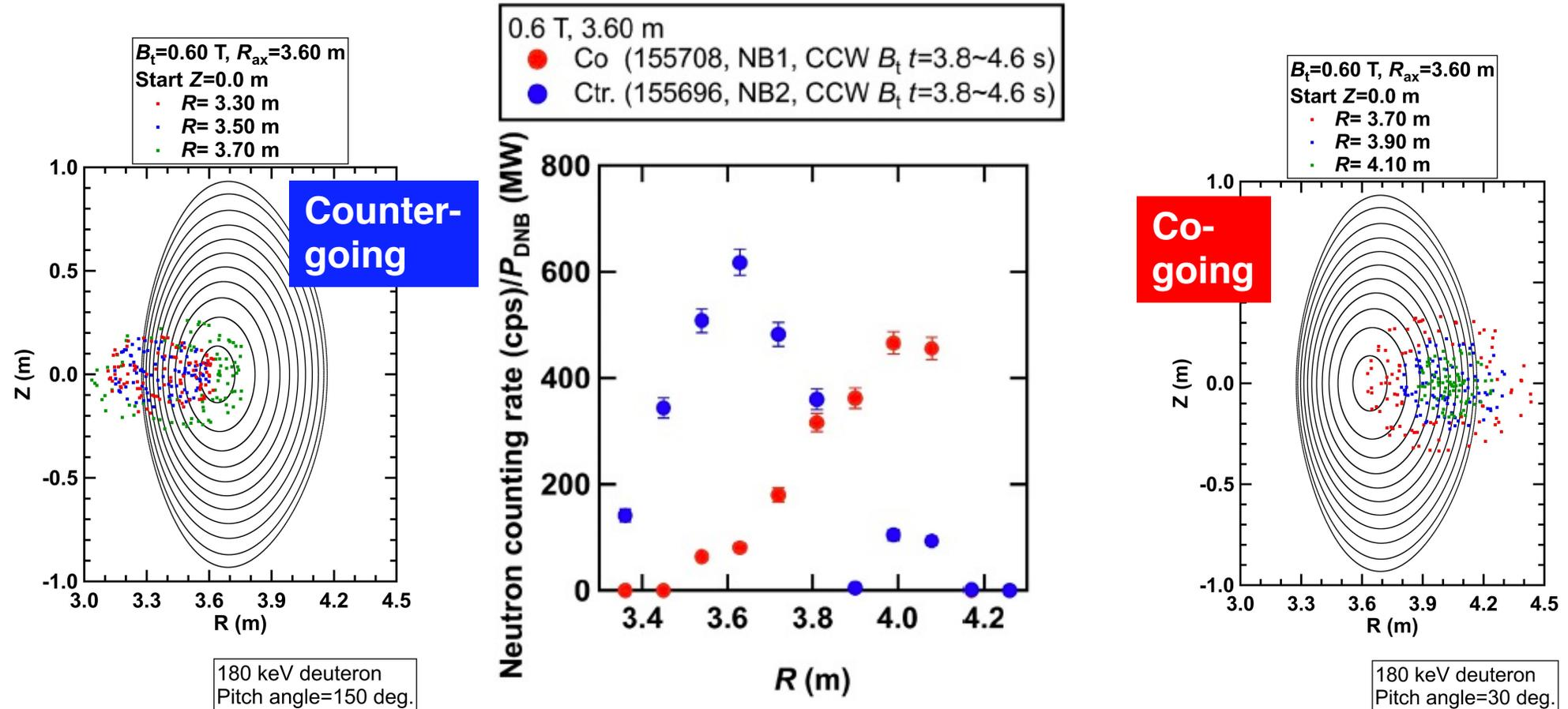
Significant inward/outward shift of neutron emission profile in low- $B_t$  condition is visible as expected by means of a vertical neutron camera.
