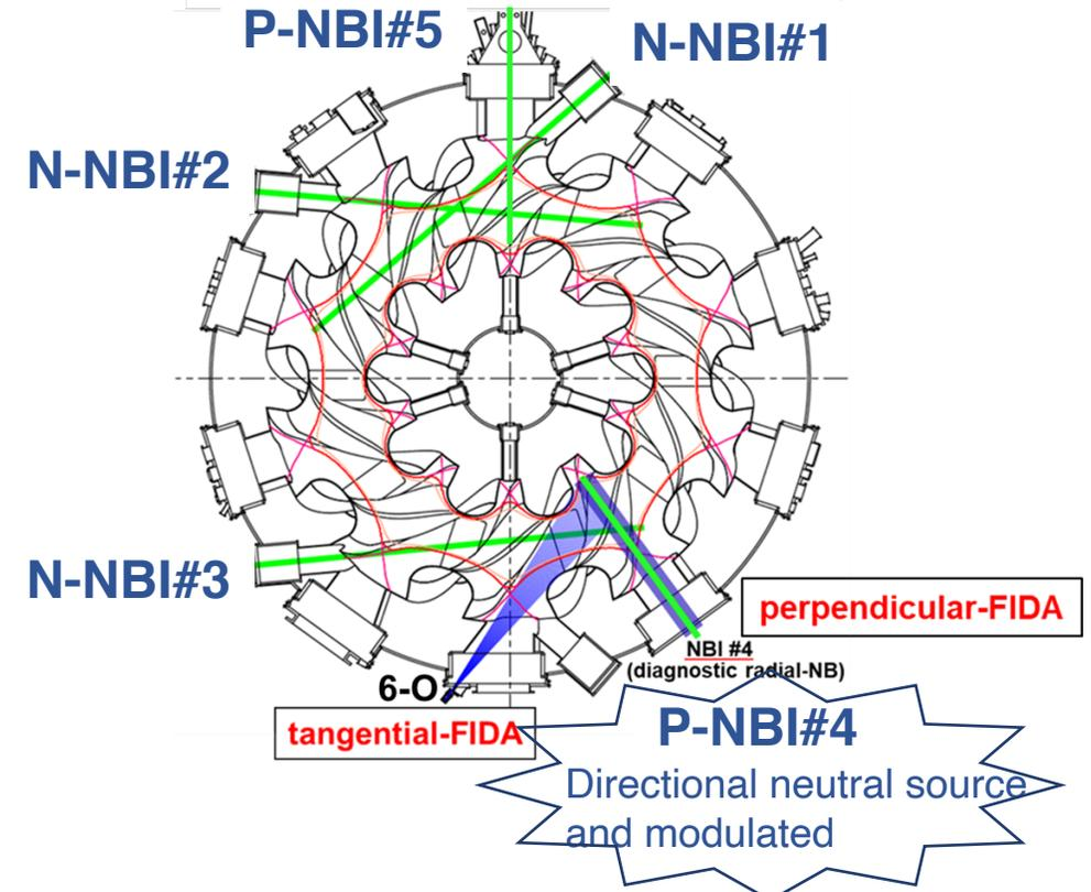
Tangential viewing geometry is suitable for observing tangentially injected beam ions parallel to magnetic field.
