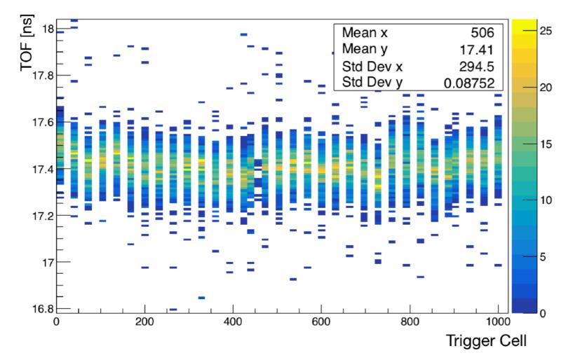
Since the time calibration is the uniform on all the buffer, the SC performance depends on the event **trigger cell** (**TC**) which is shared by its 8 channels.
