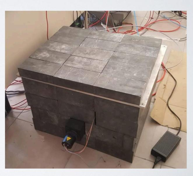
After the shielding the current dropped by a factor 2;
