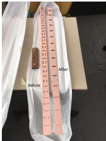
Figure 9: 1 meter long cavity prototype [3].
