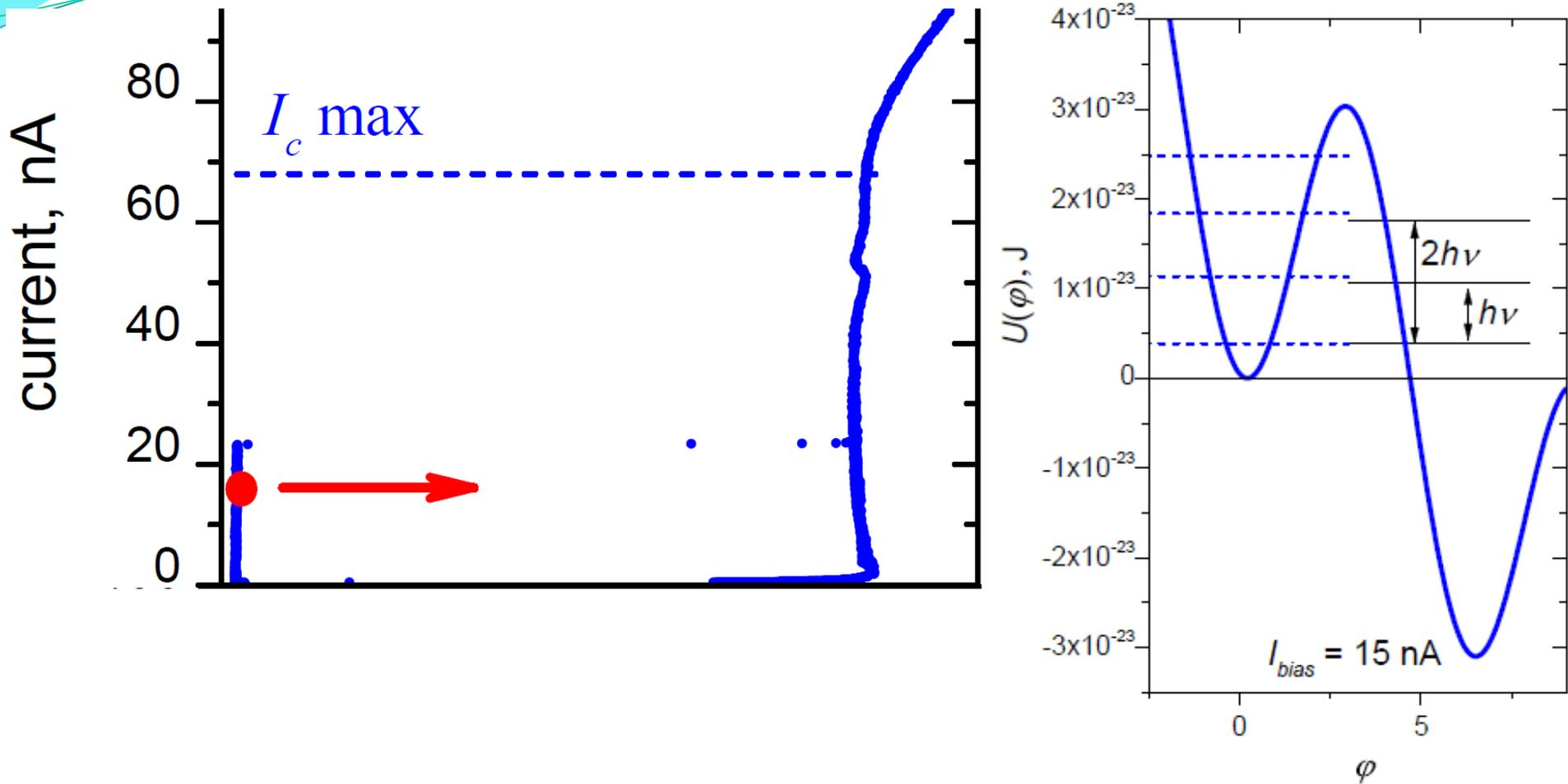
For small junctions critical current is suppressed due to MQT
