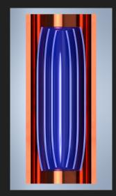
Adding more layers reduces loss along the radial direction Tapered structure reduces Ohmic losses along the axial direction
