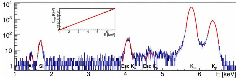
Energy calibration using O, Al, Si, Cr, Mn, and Fe X-ray lines
