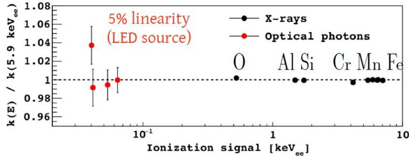
CCD linearity down to  $40\text{eV}_{\text{ee}}$  with optical photons
