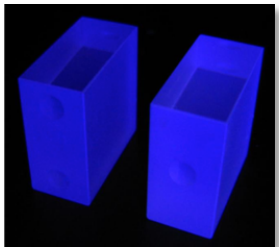
Scintillating target crystals ( \text{CaWO}_4 )
