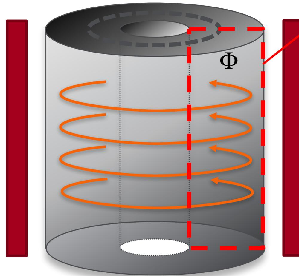
Ac B field from axions induces Flux  $F$  through dashed cross-section of the coaxial pickup
