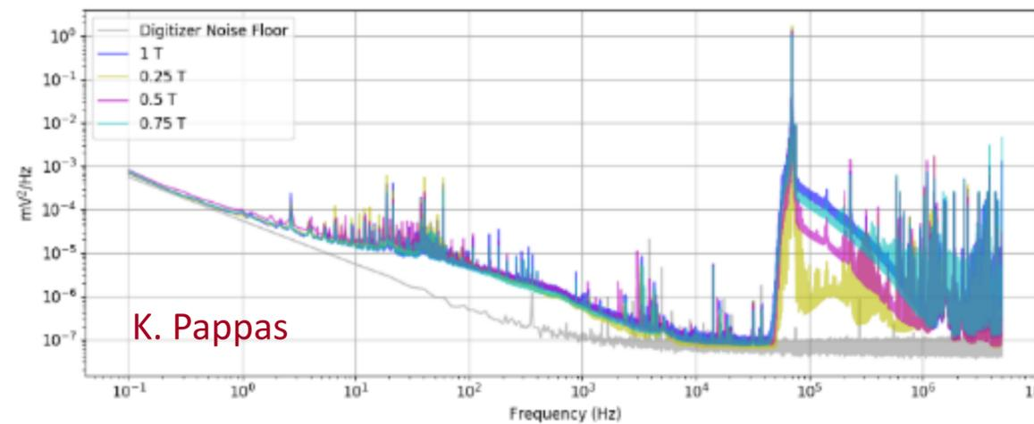
Electric Field in the DMRadio m<sup>3</sup> Coaxial Inductor
