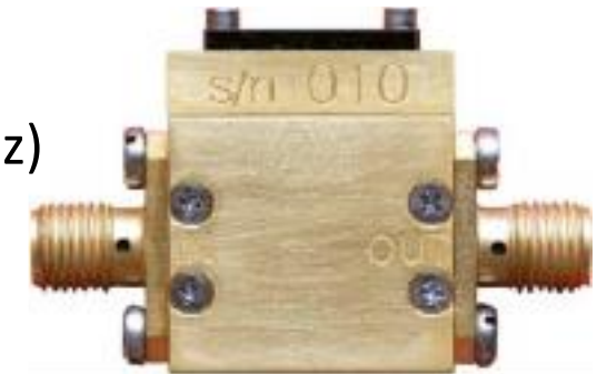
Low-noise cryogenic amplifier (noise temperature 5 to 6 K)
