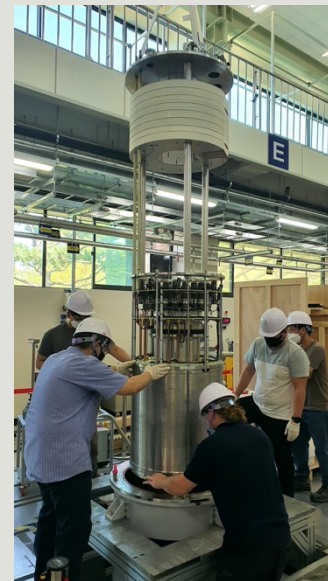
Magnet inserted in dewar at LVP Hall
