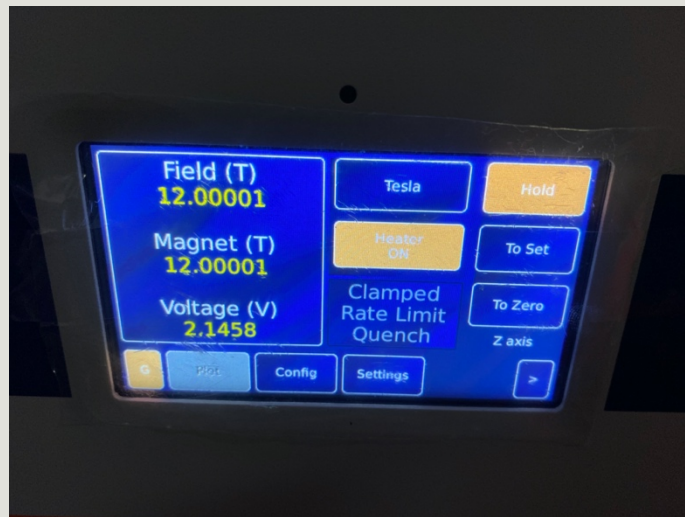
12 T shown in Magnet (T) for both driven (left) and persistent (right) mode
