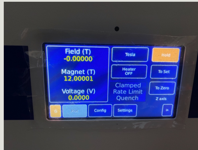
12 T shown in Magnet (T) for both driven (left) and persistent (right) mode
