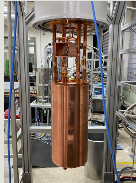
Resonant Cavity Copper tuning rod ID 262 mm, Q_0 \sim 100,000
