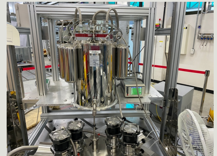
Reliquefier in operation
