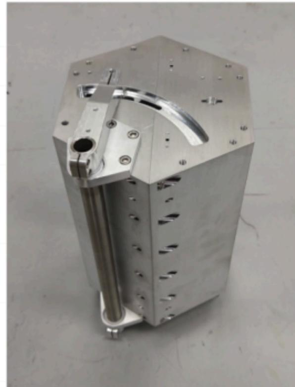
Array with fully assembled tuning system
