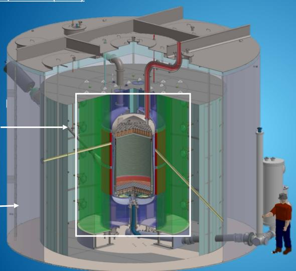
Outer veto detector: Gd-doped liquid scintillator
