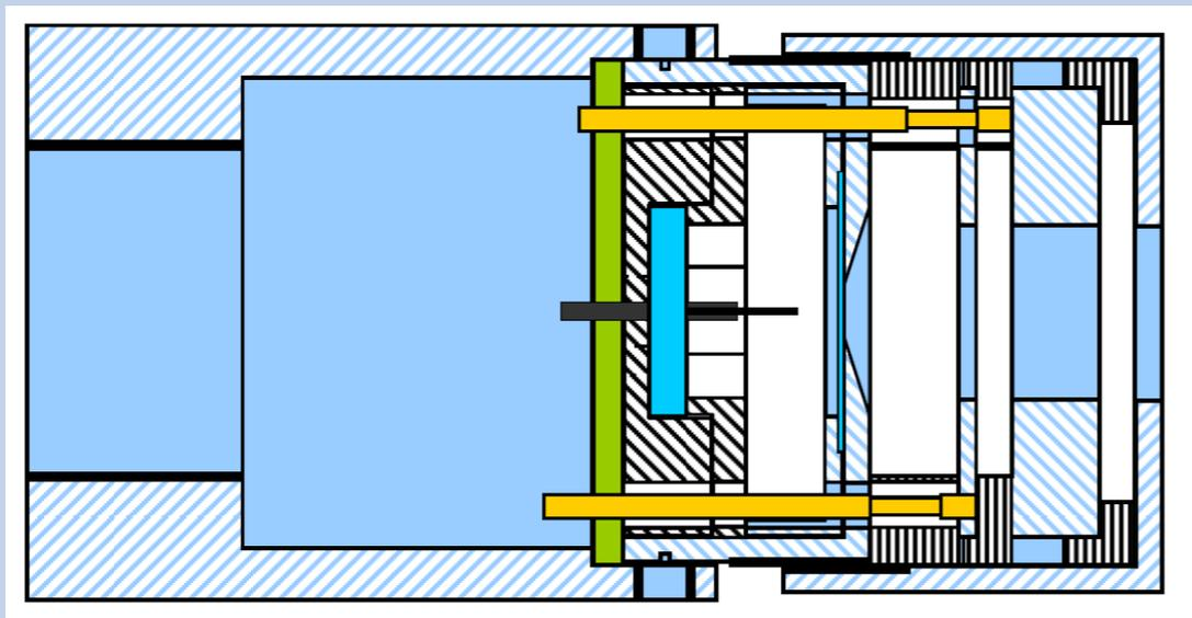
Mechanical design & working principle of a previous (2014) e-gun for plasma chambers
