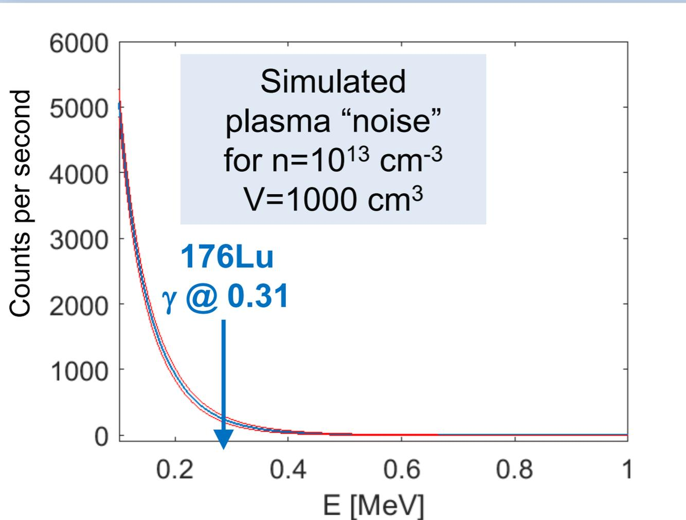
"Noise" spectrum scaled to detection efficiency (14 Ge) in order to evaluate the run-time to have Signal/Noise  $>3$
