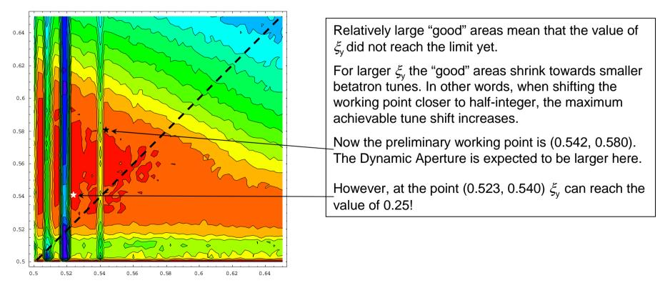
Luminosity contour plot vs. the betatron tunes. <u>Parameters as of December 2006</u>,  $\xi_y=0.17$ . In the red areas the luminosity exceeds  $10^{36}$  cm<sup>-2</sup>c<sup>-1</sup>.
