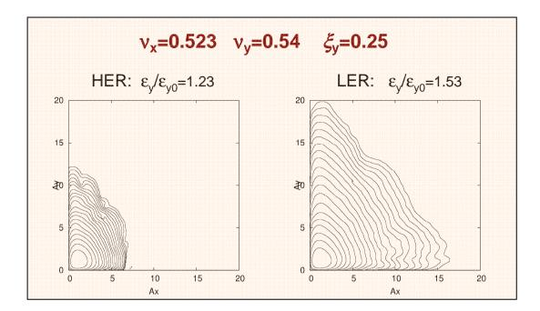
Asymmetry between LER and HER results in the different beam-beam tune shift limits.
