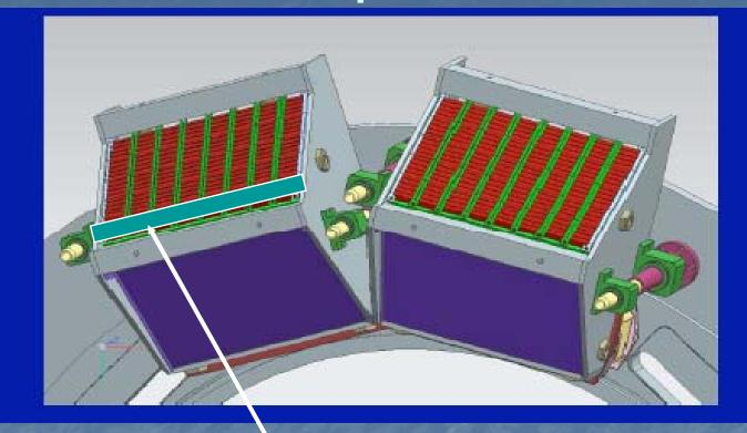
Long boards : 128 channels . Mechanical issues for a precise adjustment base to base. This high granularity has a impact in case of failure. (calculation?)
