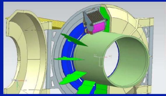
Electronics is split in two parts : - one directly mounted on the PM base receiving the PM signal and processing it with TDC/ADC - the other one concentrates and pack all the channels to send data to the DAQ
