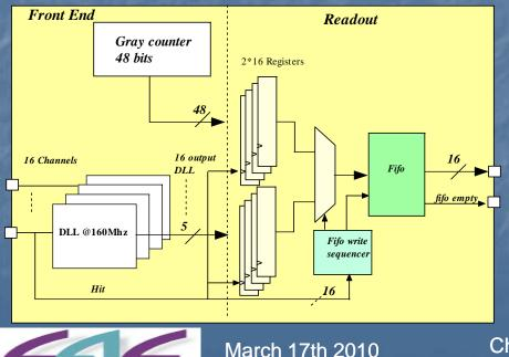
• Keeping the Gray counter inside the ASIC with an output bus width set by user in order to reduce the amount of data to be transferred. The Gray counter is duplicated inside the associated PGA.
