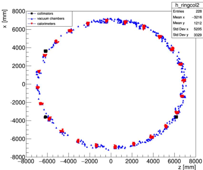
Collimators can be hit more than one time before the muon exits from the storage ring.
