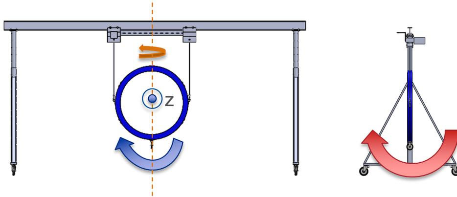
The problem of a lifting system that uses chains are oscillations: the use of two trolleys limits oscillations around vertical axis and z-axis but not around the I-beam axis
