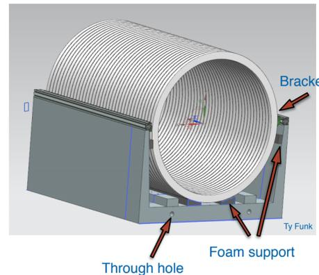
Conceptual design of the storage. From *T-Tracker assembly*, G. Gallo et al., 09/11/2018
