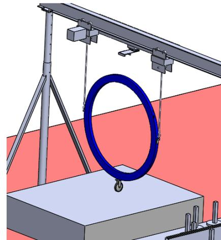
3) Motorized trolley moves the plane to the other table. The plane is lowered and the locking mechanism is disengaged.
