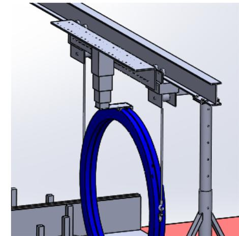
**Larger distance between trolleys** to reduce oscillation around z-axis
