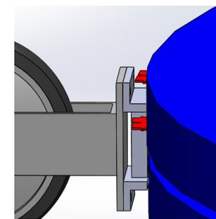
3D views of the connections: wheel – plane (on the left); wheel – station (on the right). Ears in red.
