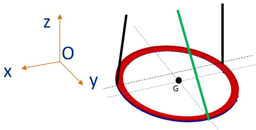
Both plane and station have **two lifting points** and a **third flange** at the bottom, needed for the correct installation in the frame.
