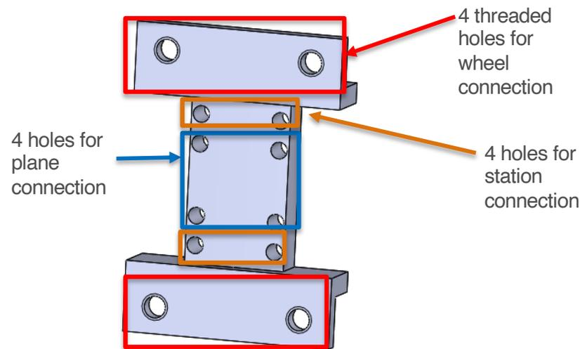
Conceptual design of the flange adapter
