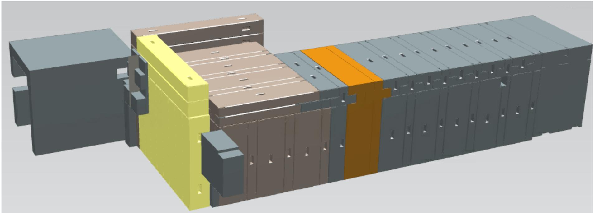
Position of the West Wall Shielding in the Upstream External Shielding subassembly.
