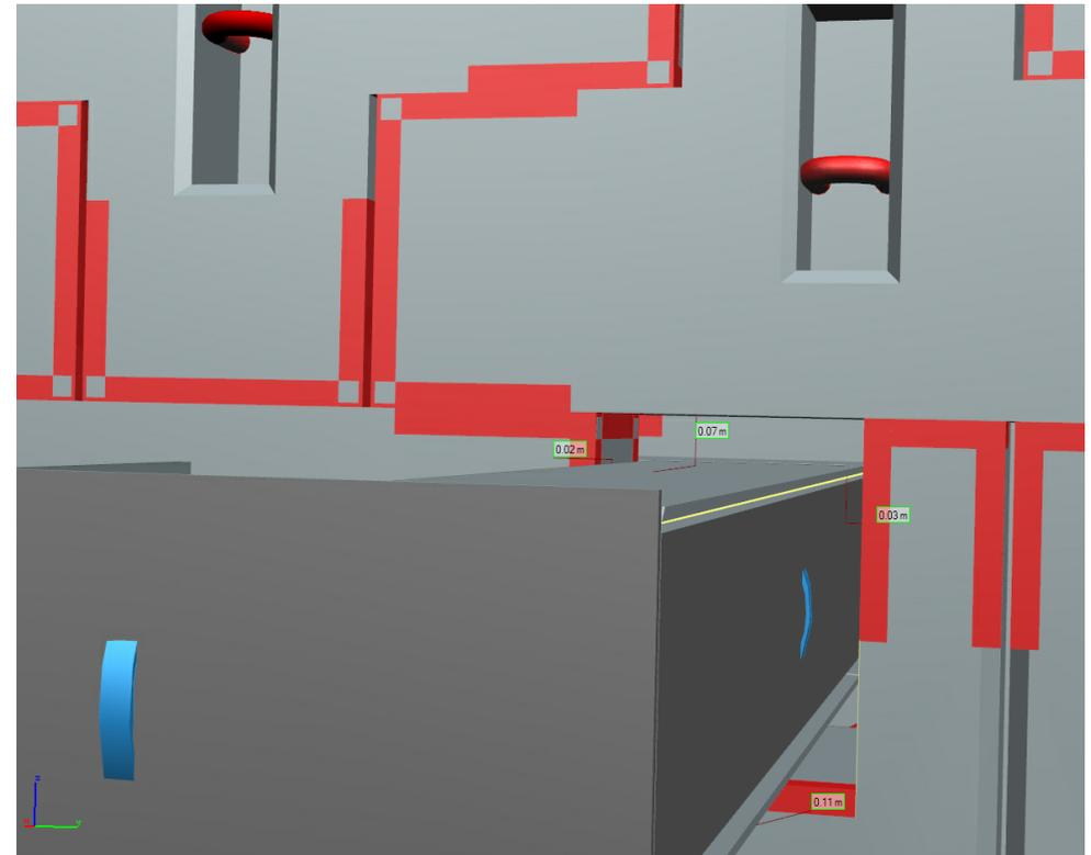
Pipe within south wall of the Downstream External Shielding .
