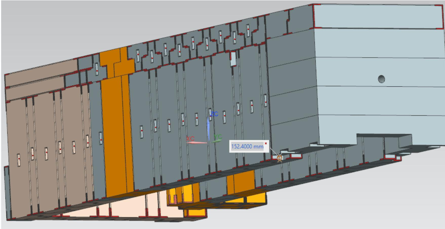
Gap Between the bottom face of the lower block of the End Cap Shielding, CU2-194, and the floor is (6") bigger than the elevation of the line of force of the pulling mechanism (4,75")
