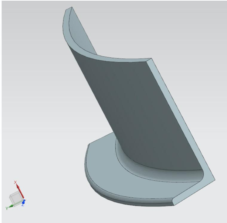
Cable Protection Brackets. Inserted into the model to be sure that the cables don't unplug while pushing out the four inspection panels.
