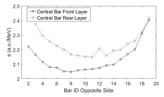
The linear parameter reproduce the trend of the total collected signal, so it is not expected to be constant along the bar.
