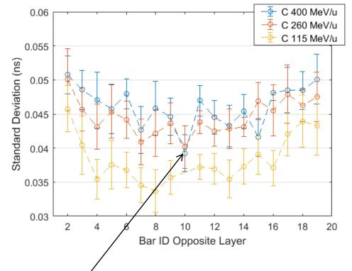
No difference in time resolution between two bars read-out by the same DRS, and bars connected to different boards. Inter-board alignement recovers completely the clock skew.
