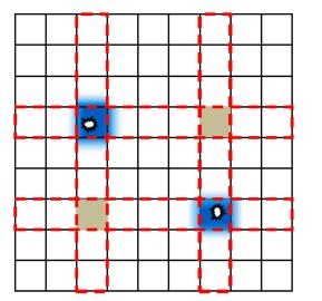
Multiple hits can be disambiguated by comparing the timestamps of the two sides of the triggered bars
