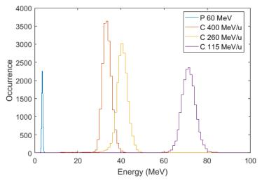
The energy resolution is expressed as the ratio between the standard deviation of the distribution and its center
