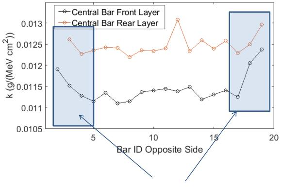
At the two edges the parameter seems to increase (SiPM saturation effect?)
