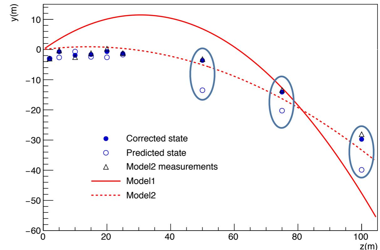
$$\text{Model2: } g = -4.91 \text{ m/s}^2 ; v_{y0} = 3 \text{ m/s} ; v_{z0} = 23 \text{ m/s}$$
