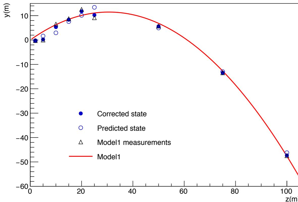
$$\text{Model1: } g = -9.81 \text{ m/s}^2 ; v_{y0} = 15 \text{ m/s} ; v_{z0} = 20 \text{ m/s}$$
