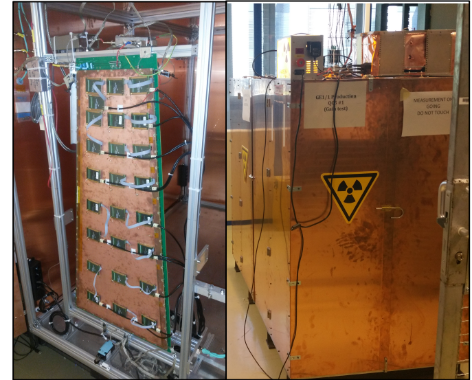
Aging setup in the GE1/1 production lab.
