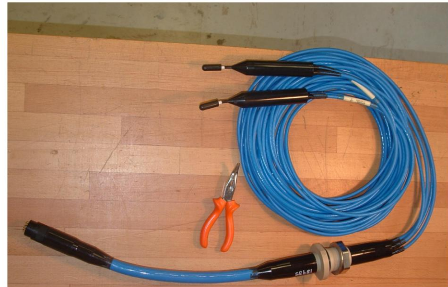
Hydrophone assembly realised by SEACON on INFN request
