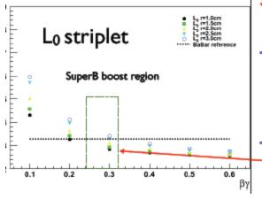
Sustainable background hit rate (radius) depends on technology: striplets vs pixel area and readout chip.
