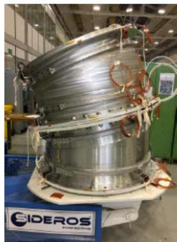
Figure 7.1: (Left) The first superconducting unit of the Mu2e Transport Solenoid composed of one single module delivered to FNAL in 2018 from ASG Superconductor in Genova (Italy); (Right) The second unit composed of two modules delivered to FNAL in 2019.
