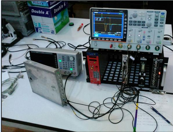
**TDC Calibration test setup**
