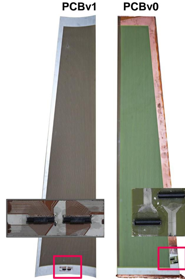
To minimize signal reflections, the stripline impedance must be controlled up to the ASIC.
