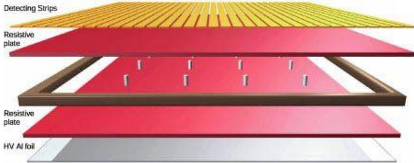
**Gas mix: 95.2% C<sub>2</sub>H<sub>2</sub>F<sub>4</sub>, 4.5% i-C<sub>4</sub>H<sub>10</sub>, and 0.3% SF<sub>6</sub>**
