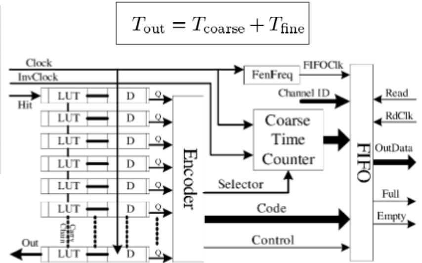
The Front-End Electronics Board (FEB) that hosts one PETIROC ASIC and the FPGA that includes the TDC and the schematics of the PETIROC ASIC
