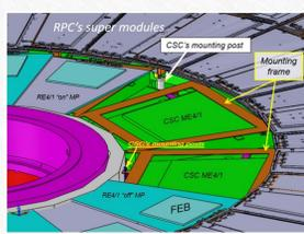
Schematic view of installation of the RE4/1 chambers
