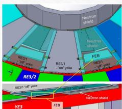
The RE3/1 chambers (plot on the left) will be mounted directly on the endcap yoke 3 (YE3) iron disk using the foreseen mounting points threaded into the yoke steel. They will cover the circular neutron shielding attached to the inner part of YE3 and reach the cylindrical neutron shielding surrounding the flange that separates the yokes YE2 and YE3. The FEBs (Front-End Boards) will be mounted behind RE3/1 chambers.
