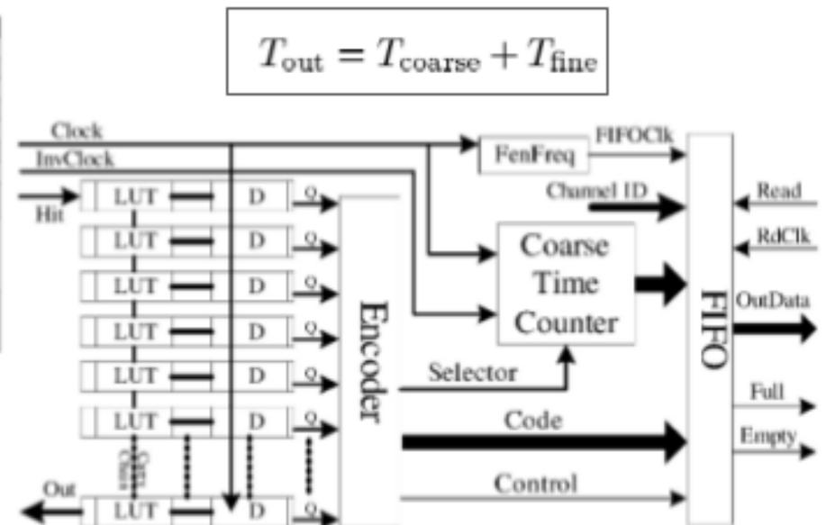
Block diagram of the time-to-digital converter implemented in a single FPGA device.
