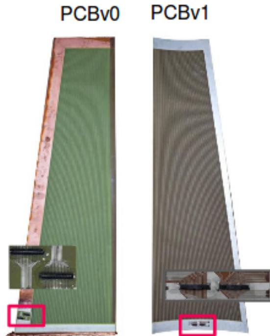
PCB with 48 (v1) or 44 (v0) strips to instrument half an iRPC chamber with connectors placed on the high eta region:
