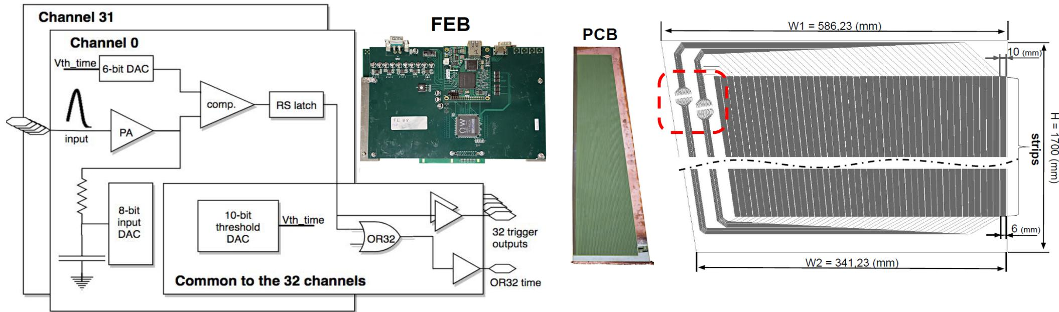
The Front-End Electronics Board (FEB) that hosts one PETIROC ASIC and the FPGA that includes the TDC and the schematics of the PETIROC ASIC [3]. (left) Photograph and dimensions of a prototype pickup-strip PCB. (right)
