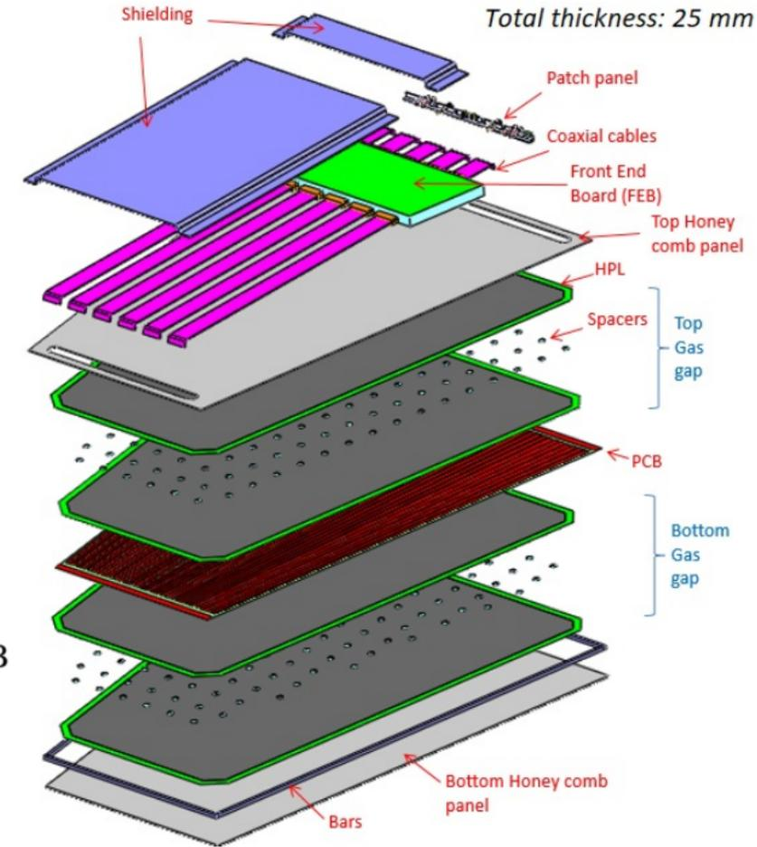
iRPC design including the readout electronics
