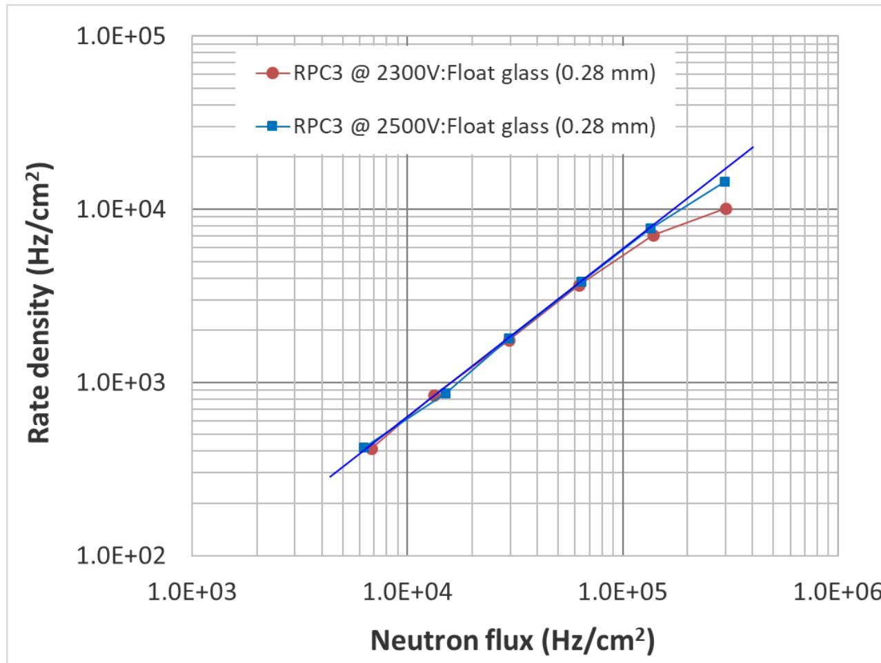
Increasing HV from 2300 V to 2500 V, maximum rate increases by a factor of  $\sim 2$
